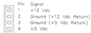
Figure 11-4. Fixed Disk Drive Power Cable Connector
