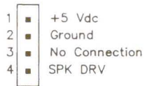
Figure 2-67. J109 and J110, Fixed Disk Drive or Fixed Disk Drive Back up Power Connector
