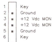
Figure 2-26. J112, COMPAQ PORTABLE 286 Monitor Connector
