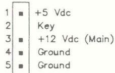
Figure 2-33. J111 and J112, COMPAQ DESKPRO 286 Diskette Drive Power Connectors
